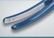
One of the instrument's jaws features ceramic pins that ensure a defined distance between the jaws over their entire length, thus preventing a short. Besides, the pins prevent tissue slippage as well.
