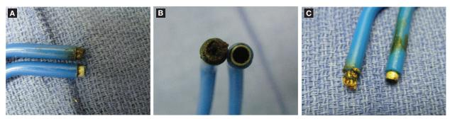
Figure. A: Photo shows two suction cautery tips after 30 seconds of cauterizing bovine renal tissue. The instrument on the bottom is coated with Electro Lube. B: Another photo shows two other tips after 30 seconds. The coated tip is on the right. C: Tips are seen after 60 seconds of cauterizing. The coated instrument is on the right.
